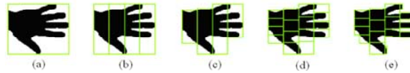
(a) Compute the bounding box B(S) of a pixel set S ; (b) subdivide S into n vertical slices; (c) compute the bounding box B(S_j) of each resulting pixel set S_j , where j=1, 2, \dots, n ; (d) subdivide each B(S_j) into m horizontal slices; (e) compute the bounding box B(S_{ij}) of each resulting pixel set S_{ij} , where i = 1, 2, \dots, m .
