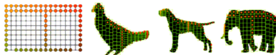
Figure 10.12: A sample points on lattice and examples of how it is mapped onto different shapes
