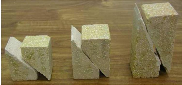
Figure 1: Specimens A after slant shear test at 1080°C
