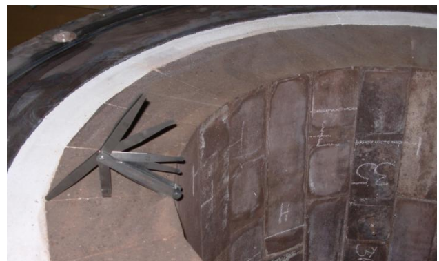
Fig. 1 Joint filler in a joint of RH-degasser snorkel.
