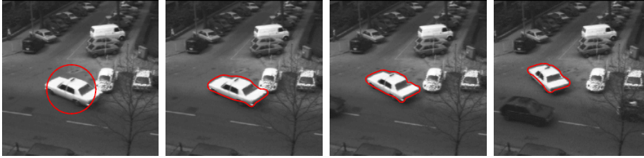
Fig. 8.3: Segmentation of a moving car with our NL-N model (3.5) and the motion distance (8.1). Initial curve (1st column) on the 1st frame and final curves (2nd-4th columns) curves on the 1st, 13th, 31th frame of the sequence are shown.
