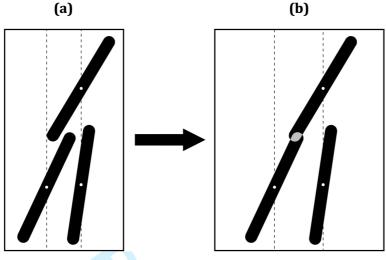
The occurrence of a molecule-molecule overlap in a system of hard spherocylinders. The system in (a) is unperturbed, while in (b) the same system is shown following an anisotropic expansion in the volume in which only the horizontal axis is scaled. Each molecules centre of mass is indicated by white dots. The presence of an overlap is indicated by the area shaded in
