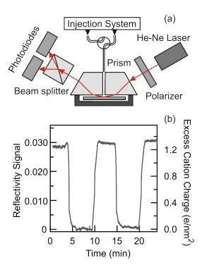
**Figure 2.** Probing ion adsorption by optical reflectivity. (a) Scheme of the experiment setup. (b) Typical experimental trace of a change between pH 10.2 and 3.0 in 200 mM NaCl solution.
