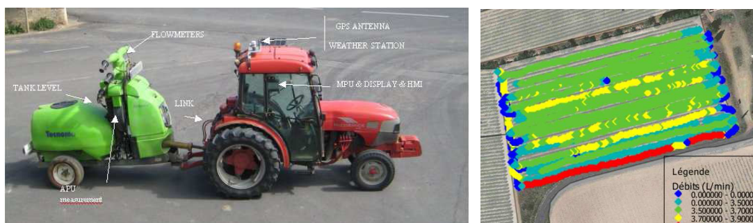
Fig 9: Traceability equipment and application map (source: cemagref 2008)
