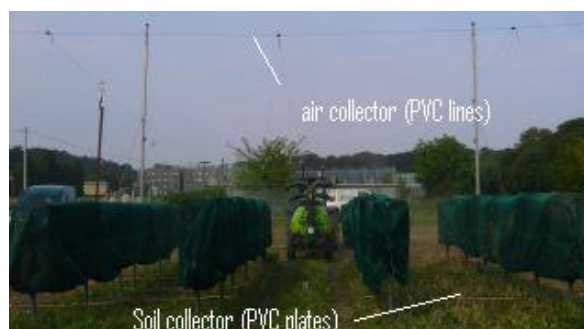
Fig 1: experimental tests on artificial vines (source: Cemagref)
