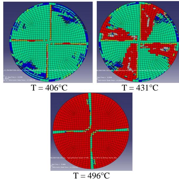
**Fig. 4 Progressive joint closure with temperature increase at the top of a fish bone bottom lining: state 1 (blue), state 2 (cyan), state 3 (green) and state 4 (red) (See Fig. 1 for state description).**
