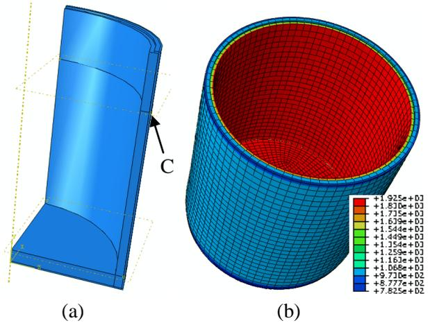
**Fig. 2 (a) One quarter of the ladle model, (b) mesh and temperature field ( $^{\circ}\text{K}$ ) of the ladle.**
