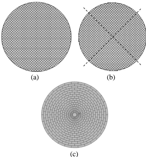
**Fig. 3 Bottom lining designs: parallel (a), fish bone (b) and radial (c).**
