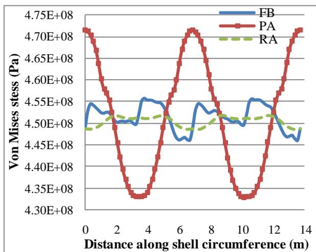
**Figure 5** Von Mises stresses in the shell along its circumference for the three models (Material I, joint thickness of 0.25mm): parallel (PA), fish bone (FB) and radial (RA).
