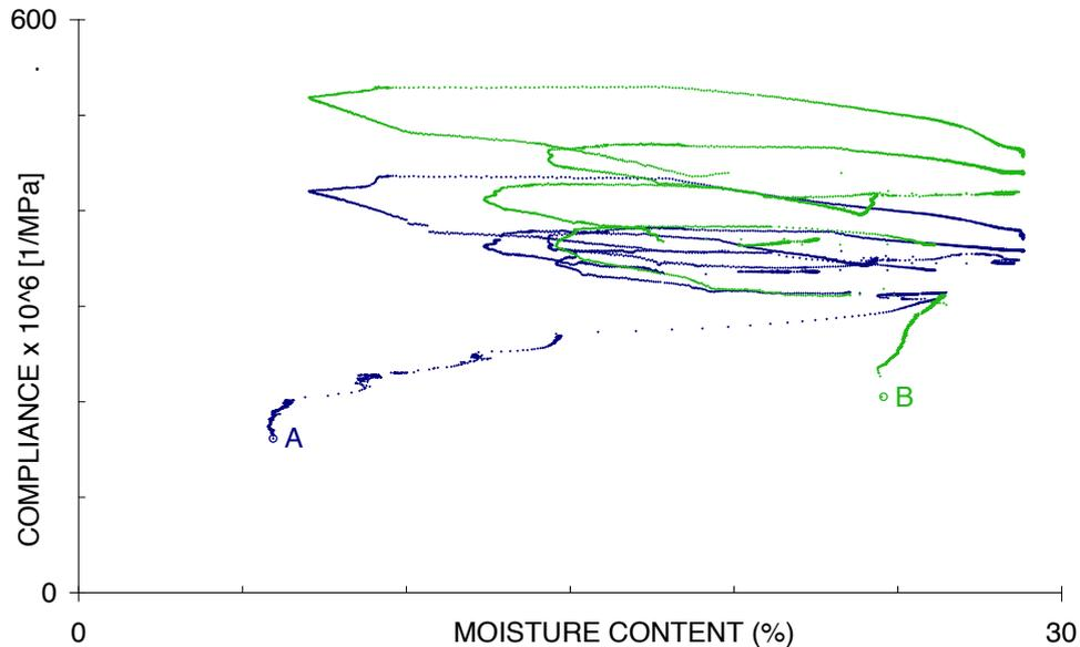
**Figure 7.** Compliance evolution for different loading history with many sorption cycle against estimated moisture content (blue : mean compliance of set A loaded at dry state , green : mean compliance of set B loaded at wet state)
