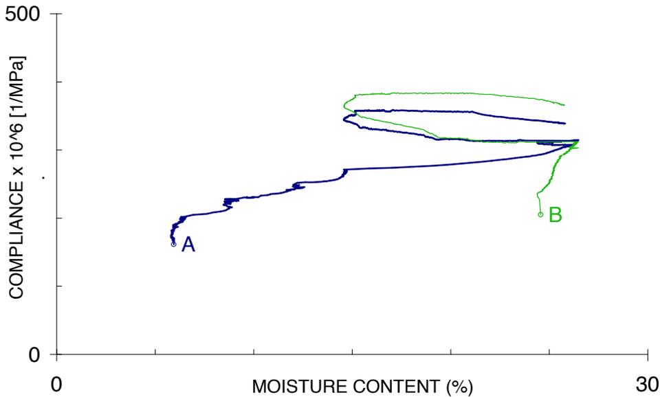
**Figure 6.** Compliance evolution for different loading history with one sorption cycle against estimated moisture content (blue : mean compliance of set A loaded at dry state , green : mean compliance of set B loaded at wet state)
