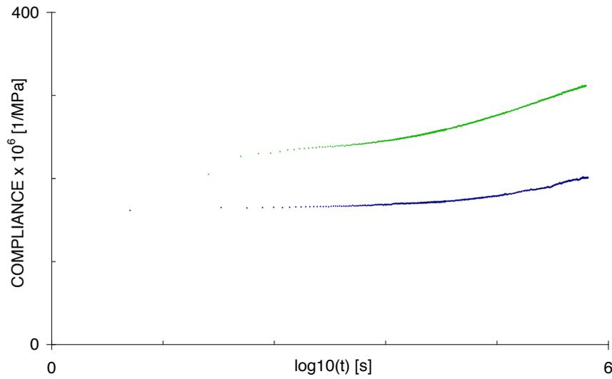
**Figure 4.** Comparison between compliance at low (blue) and high (green) moisture content against elapsed time of loading
