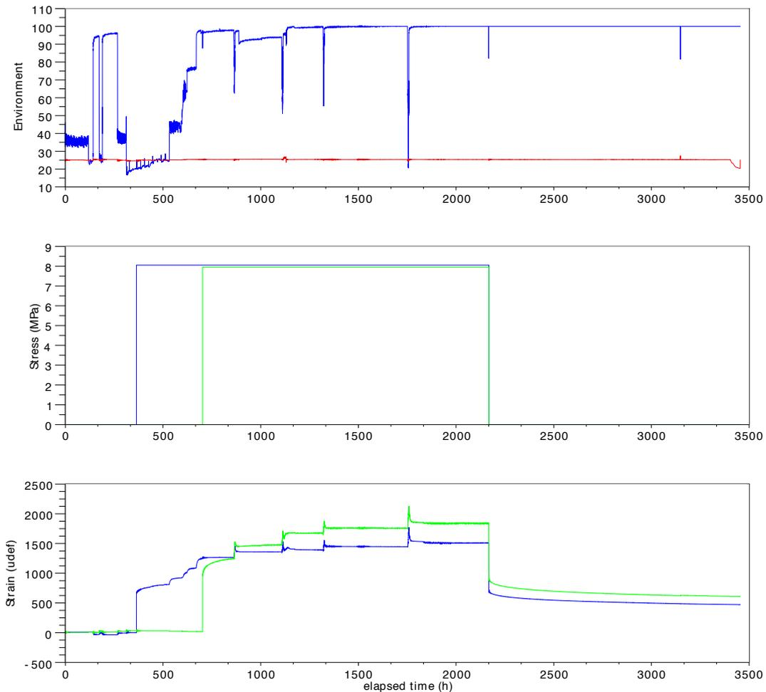
**Figure 3.** [Up] Experimental measure of the environment during the experiment (blue : relative humidity, red : temperature), [Middle] Mean stress history applied on specimens (blue : sorption A-set, green : viscous B-set), [Down] Mean strain history measured on specimens (blue : sorption A-set, green : viscous B-set).
