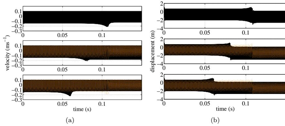
Figure 17: Case 5\_9A – Comparison of the tangential velocity and displacement on a contact node for different bases. Top: reference, middle:  $IM_2$ , bottom:  $FC_{100}^s$ . Dotted orange line is a recall of the reference. – (a) Tangential velocity on a contact node, (b) Tangential displacement on a contact node
