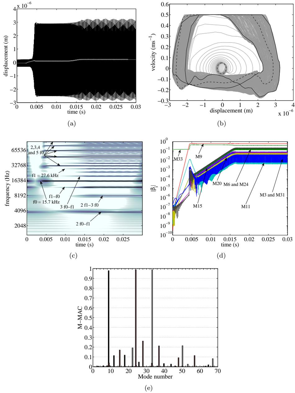
Figure 9: Case 9\_33S – (a) Tangential displacement on a contact node , (b) Phase plot – gray: complete history, black: final state, dashed black: first cycles, (c) CWT of normal velocity on contact zone, (d) Complex modal projection where “i” defines the unstable mode number for “Mi”, (e) Peak to mode M-MAC ( $\blacksquare$ : peak at  $f_0$ ,  $\blacksquare$ : peak at  $2f_0$  and  $\blacksquare$ : peak at  $f_1$ )
