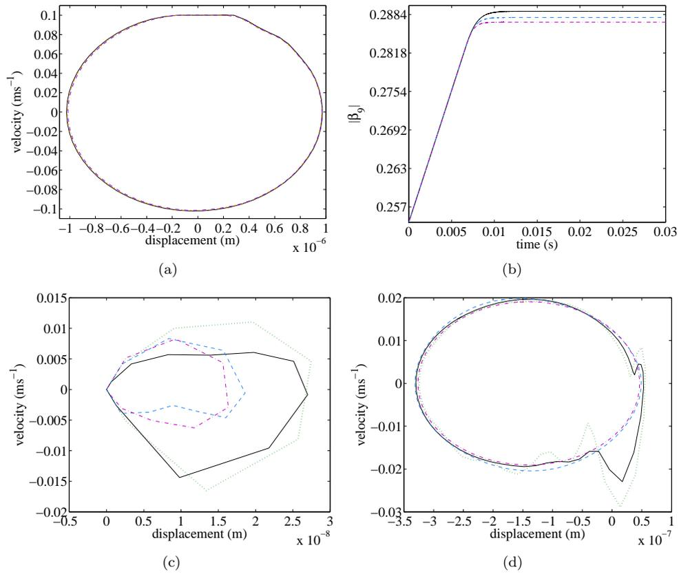
Figure 13: Bases comparison for cases 1\_9A and 1\_9S, — reference, - - -  $FC_{100}$  - - -  $IM_1$  and  $\cdots FC_{100}^s$  (only for case 1\_9S) : (a) Case 1\_9A, phase plot. (b) Case 1\_9A, modal projection. (c) Case 1\_9S, phase plot on contact zone. (d) Case 1\_9S, phase plot on an internal node.
