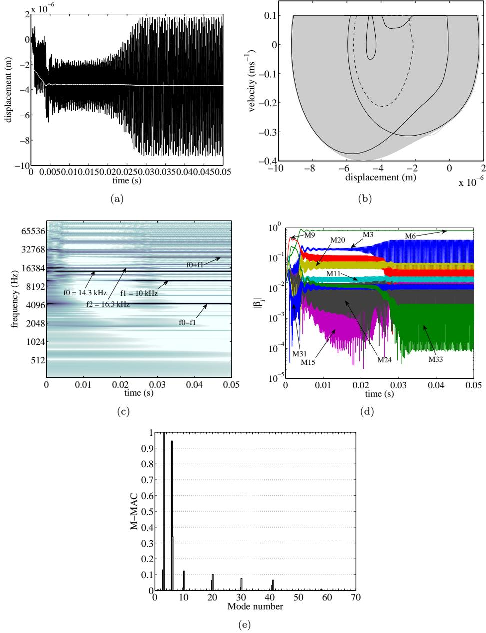
Figure 8: Case 9\_alls – (a) Tangential displacement on a contact node (gray line: mean value), (b) Phase plot – gray: complete history, black: final state, dashed black: first cycle, (c) CWT of normal velocity on contact zone, (d) Complex modal projection where “i” defines the unstable mode number for “Mi”, (e) Peak to mode M-MAC (■: peak at  $f_0$ , ■: peak at  $f_1$ )
