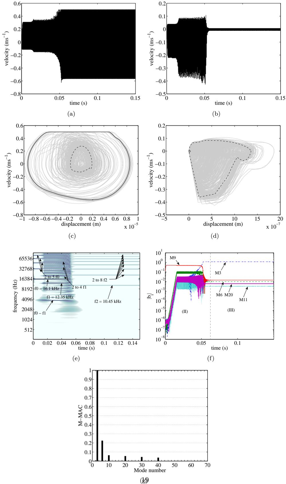
Figure 5: Case 5\_9S – (a) Velocity, tangential component on a contact node (gray line: mean value), (b) Velocity, normal component on a contact node (gray line: mean value), (c) Phase plot, tangential component, (d) Phase plot, normal component (gray: complete history, black: final cycle, dashed black: first cycle) (e) CWT of normal velocity on contact zone, (f) Complex modal projection where “i” defines the unstable mode number for “Mi”, (g) Peak to mode M-MAC at  $f_2$
