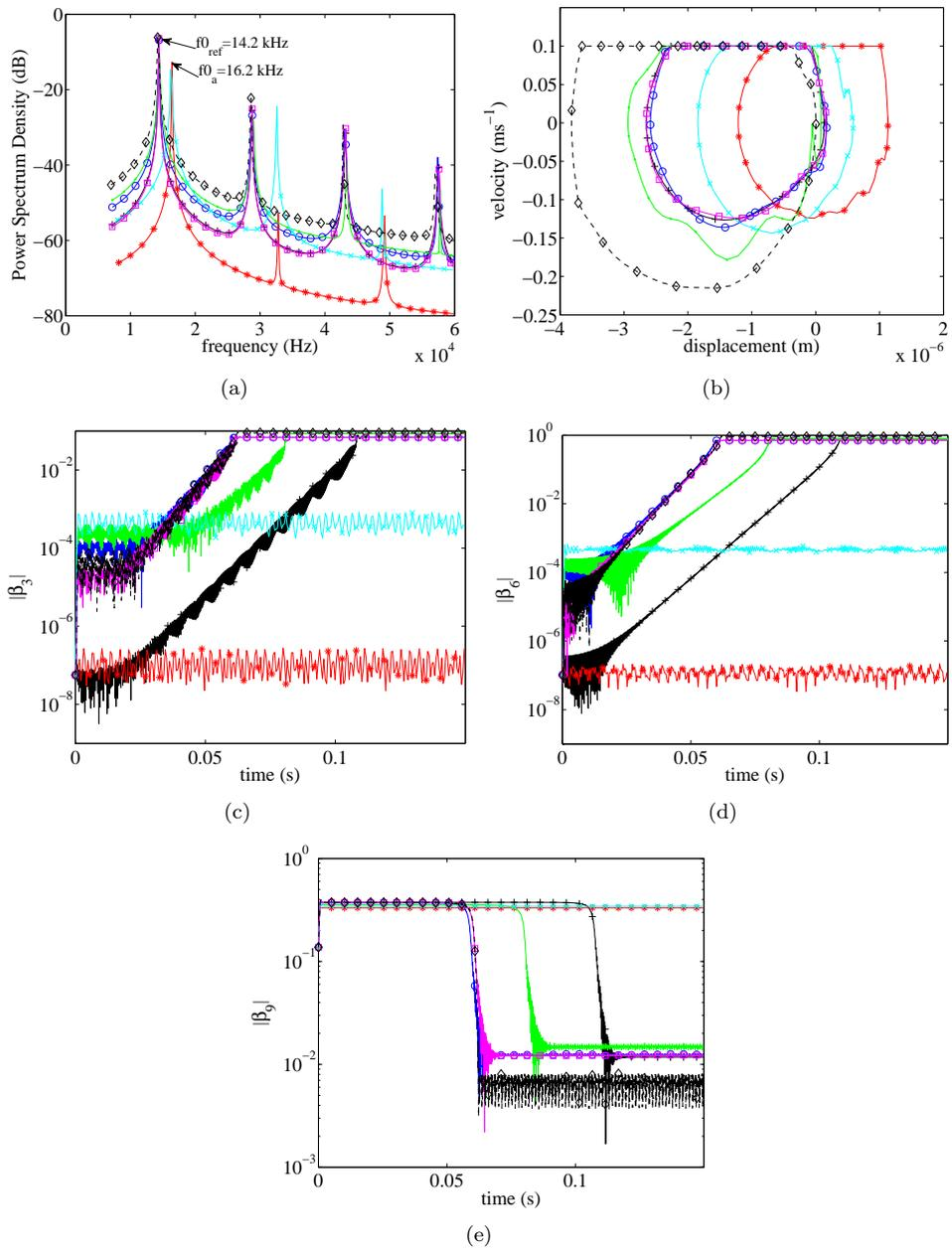
Figure 16: Bases comparison for case 5\_9A, +: reference,  $\circ$ :  $FC_{100}$ ,  $*$ :  $IM_1$ ,  $-$ :  $IM_2$ ,  $\times$ :  $IM_3$ ,  $\square$ :  $FC_{100}^s$ ,  $\diamond$  with dashed line:  $IM_2^s$  – (a) FFT of the final state, (b) Phase plot, (c) Modal projection of mode 3, (d) Modal projection of mode 6, (e) Modal projection of mode 9
