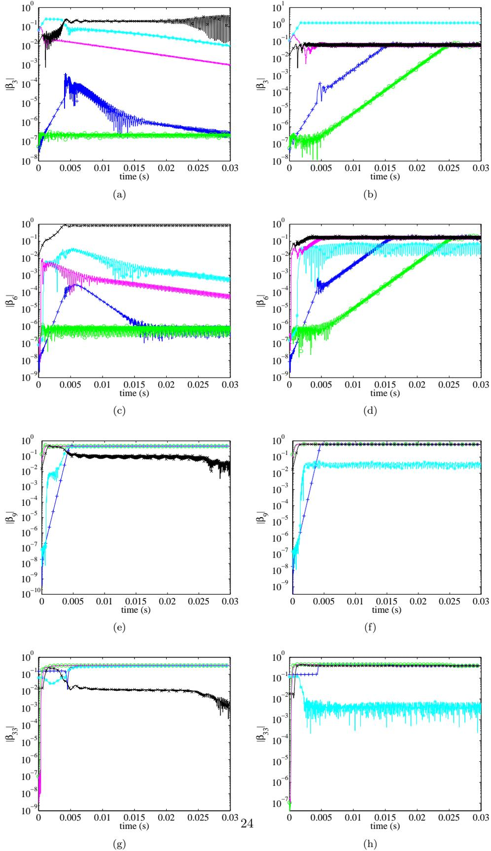
Figure 10: Existence of two final states. +: 9\_33X, o: 9\_9X, \*: 9\_3x33X, : 9\_3x9X and x: 9\_allX – (a) Mode 3 adhesion cycle, (b) Mode 3 separation cycle, (c) Mode 6 adhesion cycle, (d) Mode 6 separation cycle, (e) Mode 9 adhesion cycle, (f) Mode 9 separation cycle, (g) Mode 33 adhesion cycle, (h) Mode 33 separation cycle
