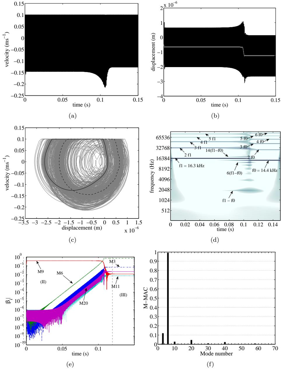
Figure 4: Case 5\_9A – (a) Tangential velocity on a contact node (b) Tangential displacement on a contact node (gray line: mean value) (c) Phase plot on contact zone (gray: complete history, black: final cycle, dashed black: first cycle) (d) CWT of tangential velocity on contact zone, (e) Complex modal projection where “i” defines the unstable mode number for “Mi”, (f) Peak to mode M-MAC at  $f_0$
