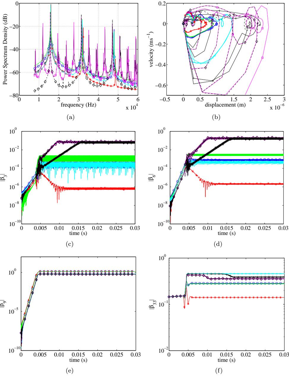
Figure 15: Bases comparison for case 9\_33S, +: reference,  $o$ :  $FC_{100}$ ,  $*$ :  $IM_1$ ,  $\cdot$ :  $IM_2$ ,  $\times$ :  $IM_3$ ,  $\square$ :  $FC_{100}^s$ ,  $\diamond$  with dashed line:  $IM_2^s$  – (a) FFT of the final state, (b) Phase plot, (c) Modal projection of mode 3, (d) Modal projection of mode 6, (e) Modal projection of mode 9, (f) Modal projection of mode 33
