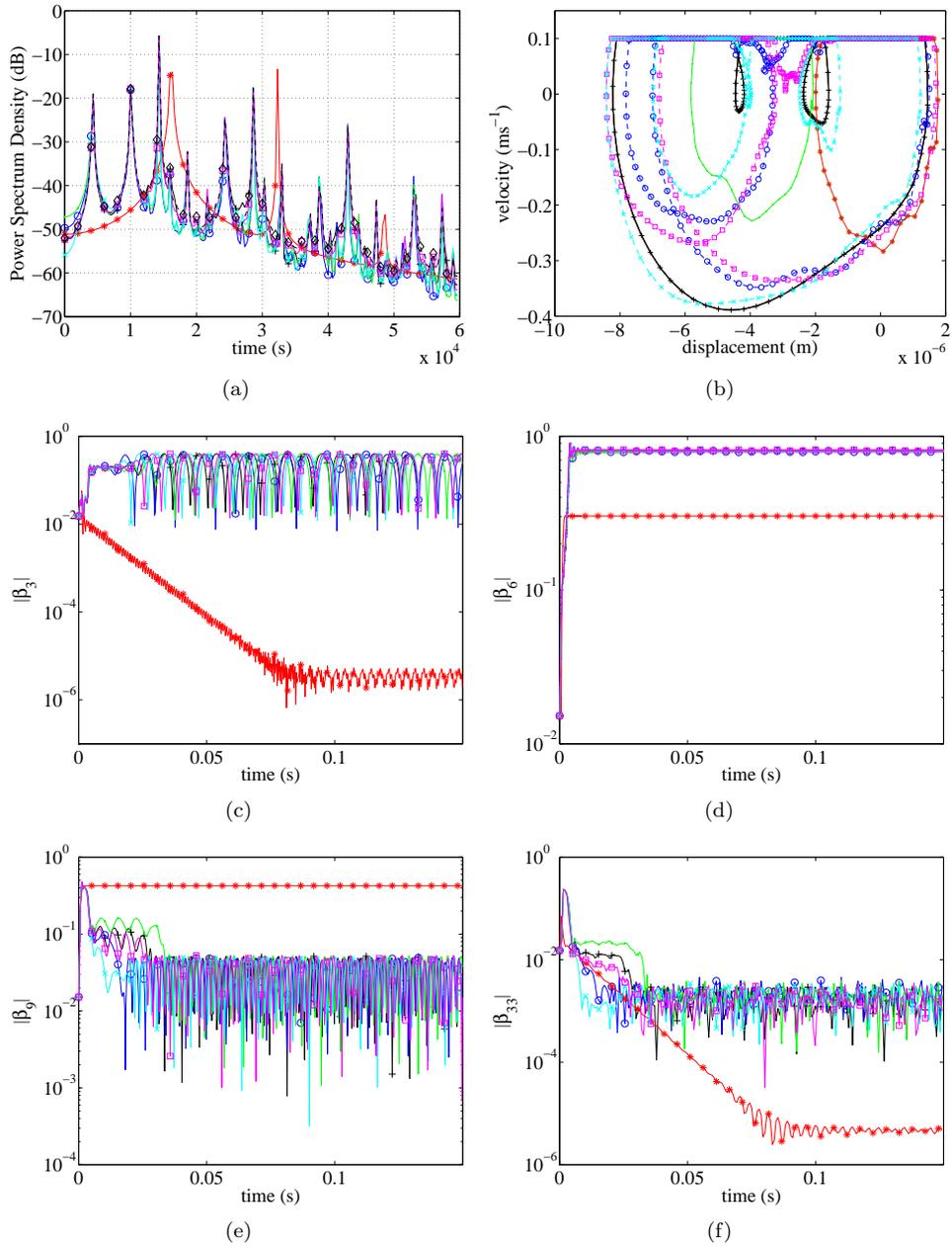
Figure 14: Bases comparison for case 9\_allA, +: reference,  $o$ :  $FC_{100}$ ,  $*$ :  $IM_1$ ,  $:$ :  $IM_2$ ,  $\times$ :  $FC_{100}^s$ ,  $\square$ :  $IM_2^s$  – (a) FFT of the final state, (b) Phase plot, (c) Modal projection of mode 3, (d) Modal projection of mode 6, (e) Modal projection of mode 9, (f) Modal projection of mode 33
