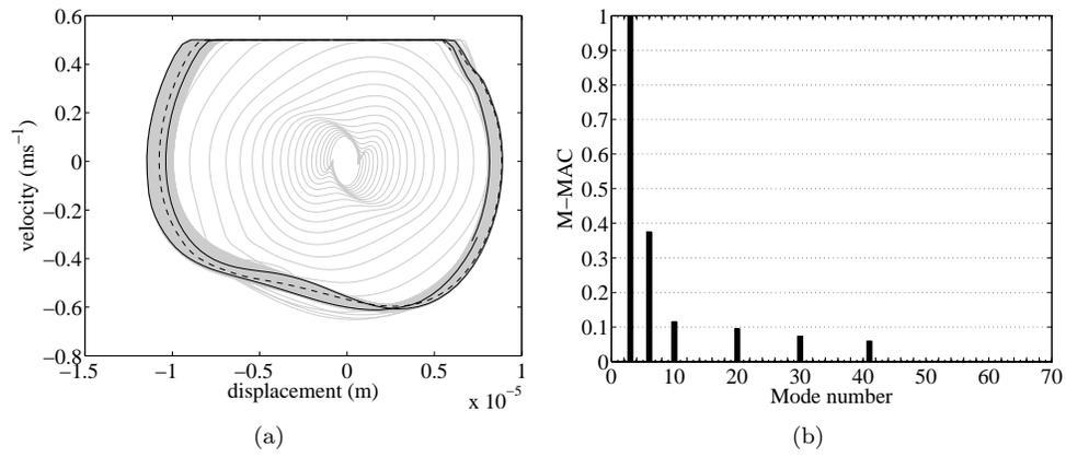
Figure 11: Case 9<sub>2</sub>×33S – (a) Tangential phase plot – gray: complete history, black: final state, dashed black: intermediate loop in final state, (b) Peak to mode M-MAC at  $f_0$
