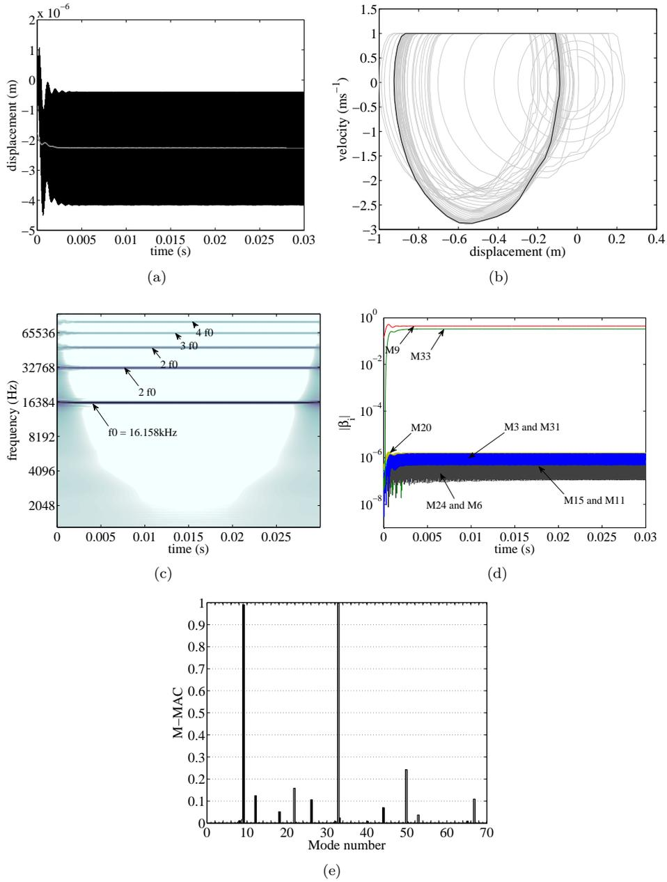
Figure 7: Case 9\_9A – (a) Tangential displacement on a contact node (gray line: mean value), (b) Phase plot, (c) CWT of tangential velocity on contact zone, (d) Complex modal projection where “i” defines the unstable mode number for “Mi”, (e) Peak to mode M-MAC (■: peak at  $f_0$  and ■: peak at  $2f_0$ )
