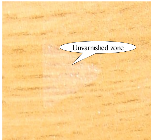
Fig.7: Intensity image of the observed piece of wood with histogram equalization for contrast enhancement
