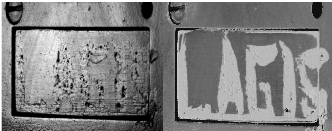
Fig.11: Detection of oil traces (text) on a metallic object (the text was written with lubrication oil for industrial tools) left: intensity image with histogram equalization for contrast enhancement; right \Delta image
