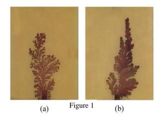
In order to obtain monopole antenna configurations, structures of Fig. 1 have been mounted vertically above a perpendicular ground plane and connected to a 3.5 mm SMA connector. The input reflection coefficients  $S_{11}$  related to  $50\Omega$  have been measured for both antenna up to 12 GHz and will be presented and discussed.
