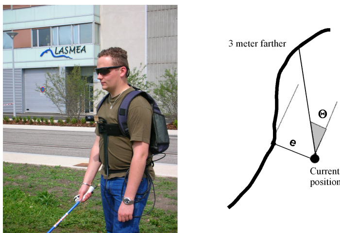
Fig. 3. Left : The pedestrian prototype with a chest mounted camera and a wearable computer in a back pack. Right : The walker is kept in a corridor along the intended path by directional prompts. His adherence to the path is defined by the angular deviation \theta for joining the route 3 meters farther from the lateral space e between current position and the nearest point of the reference path.
