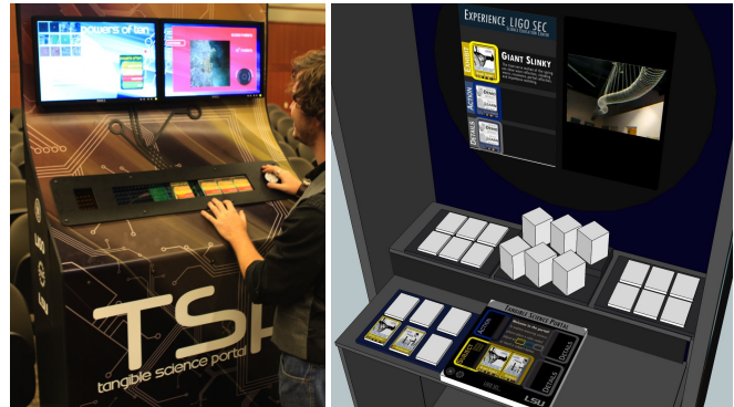
Figure 3. Mid-stage implemented kiosk + envisioned next-gen iteration. In left (implemented) kiosk, a relatively long (32x7”), black casier with captive cartouches and a haptic navigation wheel is visible as manipulated by a student. In the right (envisioned) view, five casiers on two worksurface tiers are depicted. Four are for storage (potentially sensed and illuminated) of thick (here, 3.5x2.5x2.5”) and thin DG6 (card) cartouches. The lower-center casier houses a composition of data, operation, and parameter cartouches on an iPad touch-display surface (see Figure 5 for inset).
