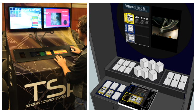
Figure 3. Mid-stage implemented kiosk + envisioned next-gen iteration. In left (implemented) kiosk, a relatively long (32x7”), black casier with captive cartouches and a haptic navigation wheel is visible as manipulated by a student. In the right (envisioned) view, five casiers on two worksurface tiers are depicted. Four are for storage (potentially sensed and illuminated) of thick (here, 3.5x2.5x2.5”) and thin DG6 (card) cartouches. The lower-center casier houses a composition of data, operation, and parameter cartouches on an iPad touch-display surface (see Figure 5 for inset).
