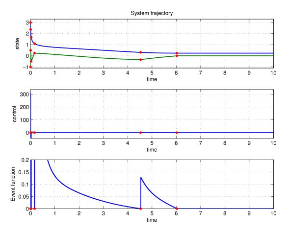
Figure 1: System (21) under event-based control with  $\alpha(x) = \beta(x) + a(x)^2$ . The red dots represent the events instants.
