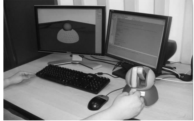
Fig. 20. Real-time indentation simulator using the Omni haptic interface.
