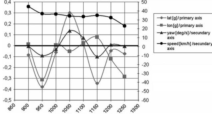
Fig. 5. Obstacle detection based on evasion maneuver.
