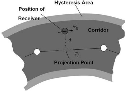
Fig. 12. Principle of trace point chain matching.
