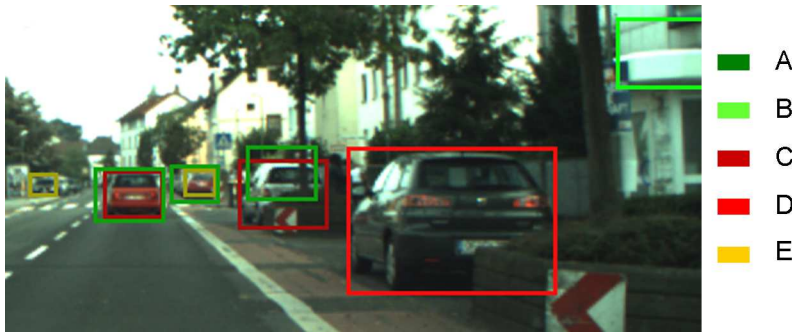
Fig. 15 Example of single-image performance evaluation. A) Hypothesis matching an annotation (true positive case) B) hypothesis not matching any annotation in the current image (false positive case) C) annotation matched by one or more hypotheses D) annotation not matched by any hypothesis (false negative case) E) annotation that is not considered due to size constraints, see text. Such annotations do not constitute a false negative case when matched by a hypothesis, but neither a true positive case otherwise.
