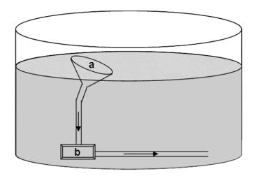
Figure 1: The experimental system constituted of a funnel (a) linked to a water pump (b) in a 300-1 sea tank.  $\rightarrow$  indicates the direction of seawater and/or contaminants through the experimental system
