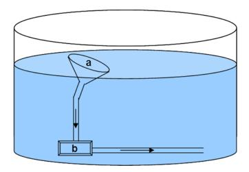
**Figure 1**: The experimental system constituted of a funnel (**a**) linked to a water pump (**b**) in a 300-l sea tank. (→) indicates the direction of seawater and/or contaminants through the experimental system
