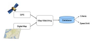
Fig. 3. Use of a navigation-based sensor. After having located the vehicle on the road network, attributes concerning the driving context are extracted from the database in order to determine the corresponding speed limit.
