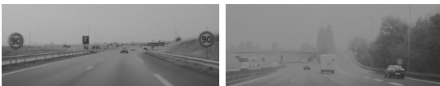
Fig. 8. Comparison of acquired images in normal (a) and in rainy (b) situations. As the presence of rain deteriorates the image quality, errors occur in the traffic sign recognition.
