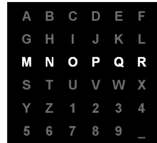
Figure 1: Classical P300 interface with the third row intensified.
