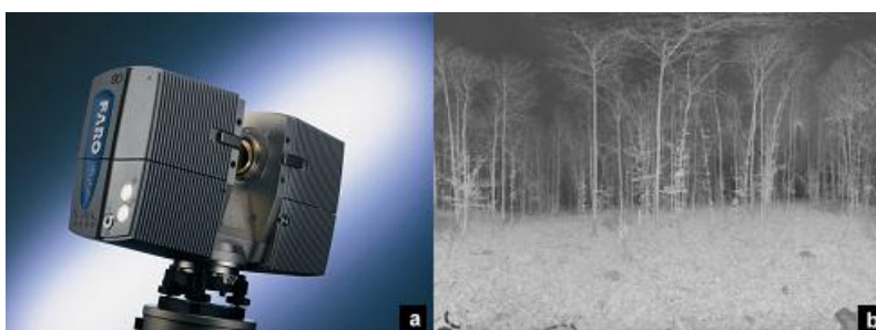
Figure 1: (a) laser scanner Faro Photon 120, (b) a 44 million points scan quick view
