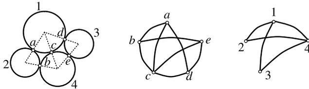
Figure 1: Left: a simple connectivity between grains (1 to 4) with potential contacts ( $a$  to  $e$ ). Middle: the corresponding dual graph. Right: the corresponding primal graph.
