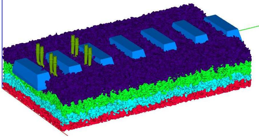
Figure 8: A railway slice of seven sleepers with tamping tines
