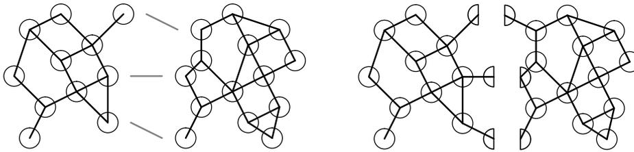
Figure 3: Primal decomposition (left) with links as interface, dual decomposition (right) with nodes as interface
