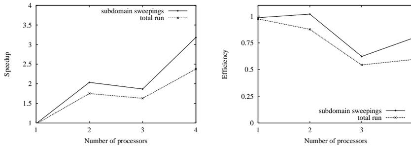
Figure 14: Performance of the parallelization with 4 subdomains
