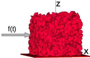
Figure 12: Sample with 2000 grains and an harmonic force
