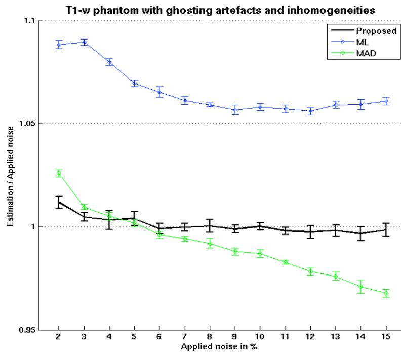
Figure 3. Results obtained by the compared methods for all the level of noise on synthetic image with ghosting artefacts and 20% of inhomogeneities.
