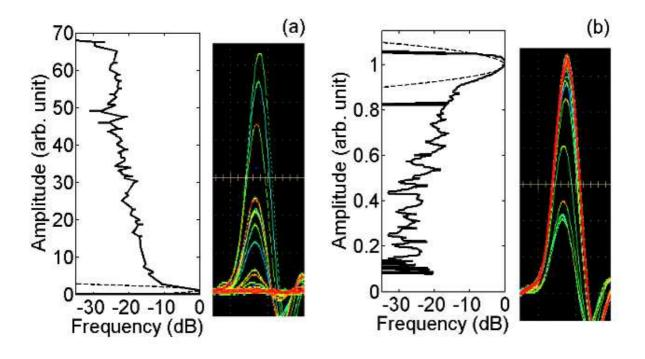
Fig. 7. Statistical distribution of the fluctuations (left, plotted on a linear scale) recorded at the output of the magnifying device, as well as corresponding electrical eye-diagrams (right). Probability and amplitude are normalized to 1 for the most likely event. The initial periodic sequence of amplitude modulation of the peak powers of the pulses is plotted in inset.
