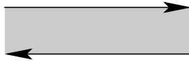
Figure 16: A straight stroke with uniform color (the shaded rectangle) would produce two line segments, one on each side (the arrows).
