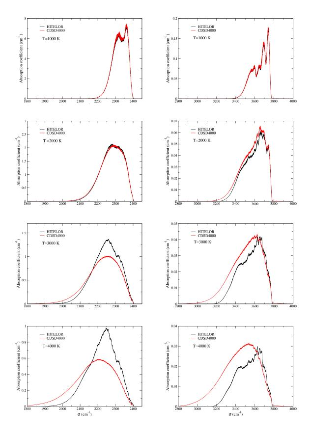
Figure 8: Pure CO<sub>2</sub> absorption coefficient at 1 atm and different temperatures.
