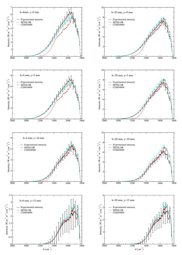
Figure 2: Experimental and theoretical line of sight integrated intensities at h=6 mm (left) and h=20 mm (right) and different distances y from plasma center; quartz tube; 2.7  $\mu$ m region.
