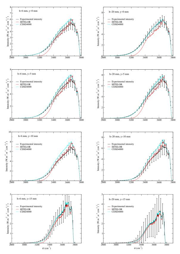
Figure 3: Experimental and theoretical line of sight integrated intensities at h=6 mm (left) and h=20 mm (right) and different distances y from plasma center; sapphire tube; 2.7  $\mu$ m region.
