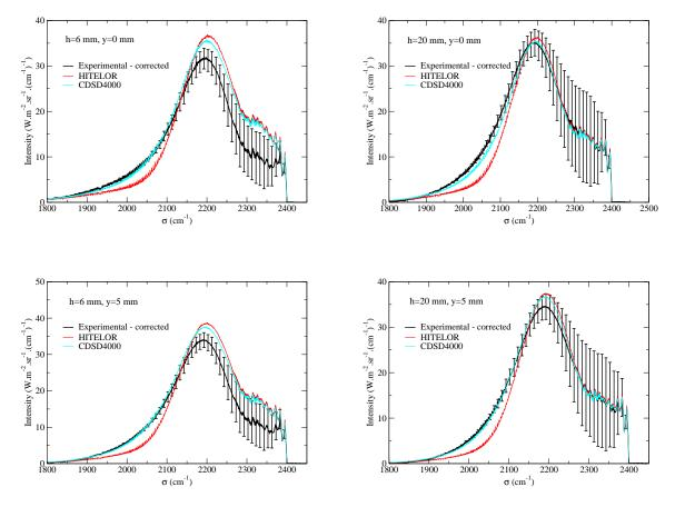
Figure 5: Experimental (corrected) and theoretical line of sight integrated intensities at h=6 mm (left) and h=20 mm (right) and for y=0 (central chord) and y=5 mm; sapphire tube ; 4.3  $\mu$ m region.
