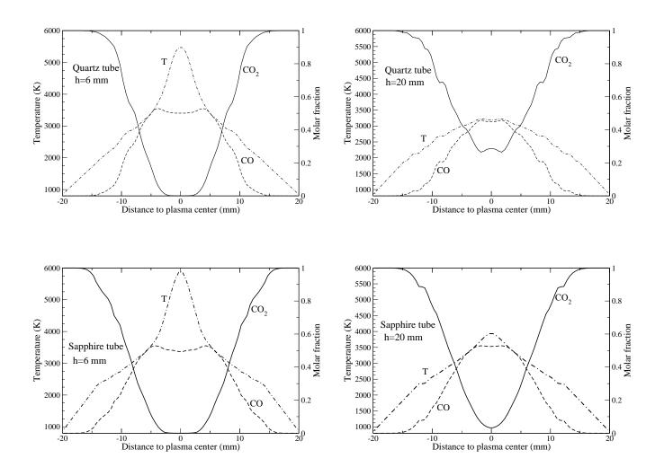
Figure 1: Temperature profiles deduced from CO normalized emission spectra with quartz and sapphire tubes at two heights h above the plasma cavity. CO and CO<sub>2</sub> molar fractions are deduced from calculations at local chemical equilibrium.
