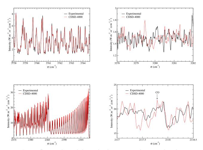
Figure 7: Comparison between high spectral resolution experimental intensities, obtained with a sapphire tube on the central chord at h=20 mm, and CDSD-4000 predictions in four selected spectral regions.
