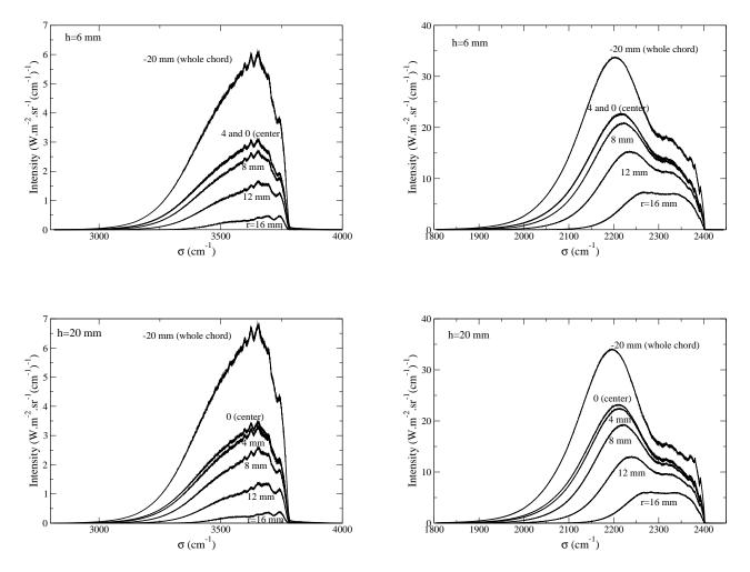
Figure 6: Partial intensities on the central chord computed with CDSD-4000 and the temperature profile obtained with a sapphire tube at h=6 mm and h=20 mm.
