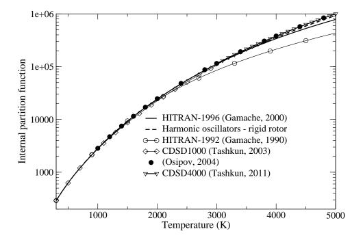
Figure 10: Internal partition sum of  ${}^{12}C^{16}O_2$  according to different calculations.
