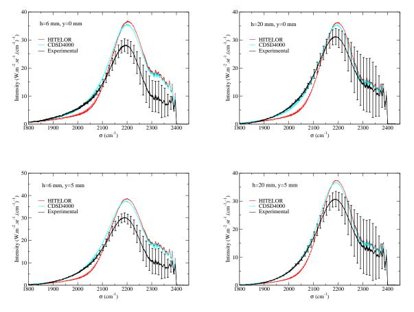
Figure 4: Experimental and theoretical line of sight integrated intensities at h=6 mm (left) and h=20 mm (right) and for y=0 (central chord) and y=5 mm ; sapphire tube ; 4.3  $\mu$ m region.
