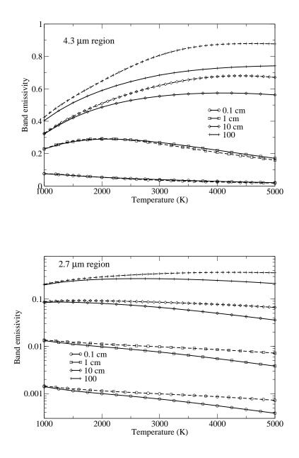
Figure 11: Total band emissivities of pure  $CO_2$  at 1 atm as predicted from CDSD-4000 (dashed lines) and HITELOR (solid lines) in the spectral ranges 1800–2450 cm<sup>-1</sup> (upper part) and 2800–4400cm<sup>-1</sup> (lower part) for different column lengths.
