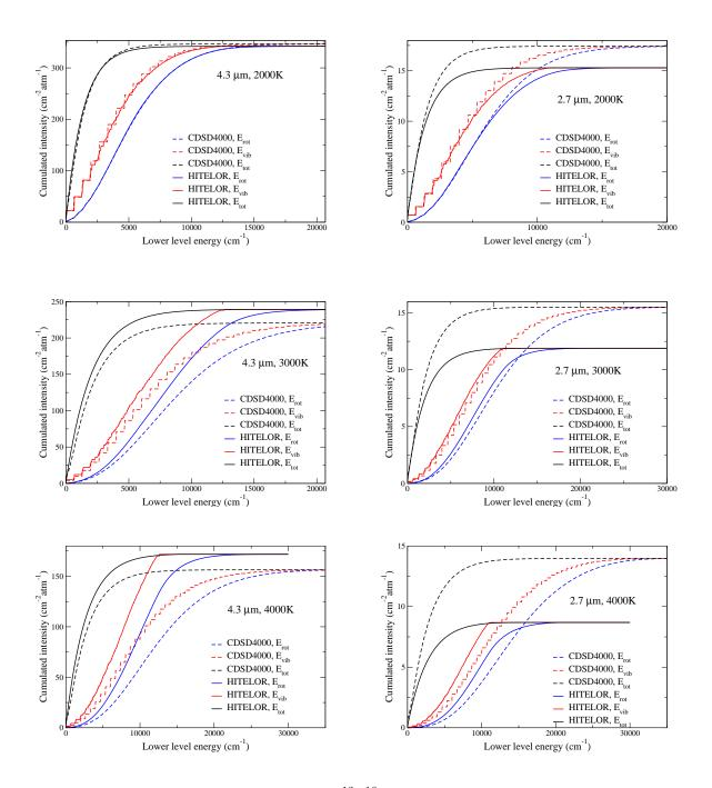
Figure 9: Cumulated distribution function of  ${}^{12}C{}^{16}O_2$  line intensities vs lower level energy in the two spectral regions and for different temperatures.
