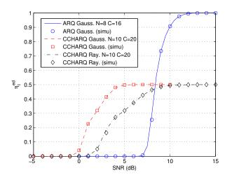
Figure 1. Theoretical and empirical efficiencies versus SNR for different types of HARQ when ED is applied.
