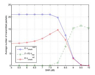
Figure 3.  $\Pi \check{n}$  and  $(1 - \Pi)\hat{n}$  versus SNR (ARQ scheme, AWGN channel, QPSK constellation, N = 14, and C = 21).
