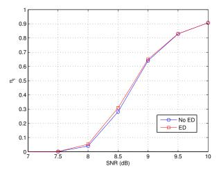
Figure 2. Efficiency versus SNR (ARQ scheme, AWGN channel, QPSK constellation, N = 14, and C = 21).
