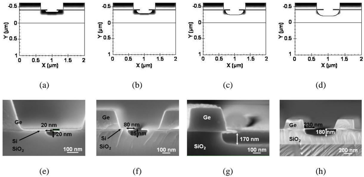
**Figure 6.** Simulated profiles of As implanted silicon dioxide etched with HF-1% for various times: (a) 2 mins, (b) 5 mins, (c) 10 mins and (d) 15 mins. (e)–(h) show the cross section SEM micrographs of the etched silicon-dioxide for the same etching times, respectively.
