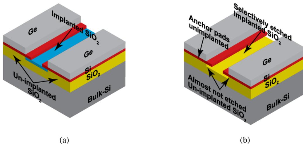
**Figure 2.** Schematics of the test structures: (a) implanted silicon-dioxide (blue region) using Ge layer as an implantation mask, the yellow region shows the unimplanted oxide region, (b) selective etching of the implanted silicon-dioxide in liquid HF solution or VHF. The openings in the germanium are larger than in the top-silicon and the anchor pads in the silicon are unimplanted due to the physical barrier to implantation provided by the germanium.
