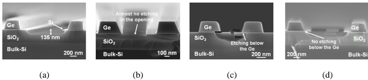
**Figure 10.** Cross section SEM micrographs of samples etched with VHF at  $55^\circ\text{C}$  (a) and (c) implanted  $\text{SiO}_2$ , (b) and (d) unimplanted  $\text{SiO}_2$ . For (a)-(b) etching is performed in a sequence of 5 etch & rinse cycles at  $55^\circ\text{C}$  with etch time of 10 mins and rinse time of 10 mins, whereas for (c)-(d) etching is performed with a similar sequence of etch and rinse cycles but with an etch time of 30 mins and rinse time of 10 mins, respectively.
