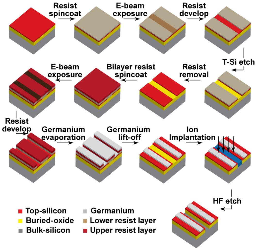
**Figure 3.** Schematic of the complete process flow.
