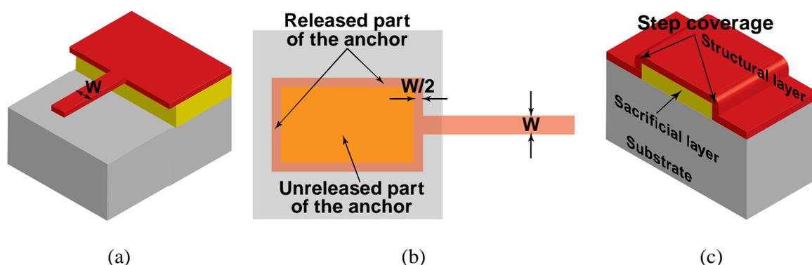
**Figure 1.** (a) Schematic of released cantilever beam, (b) underetch below the anchor pad. The width of the underetch is half the width of the released beam and (c) step coverage of structural material over a predefined sacrificial layer.
