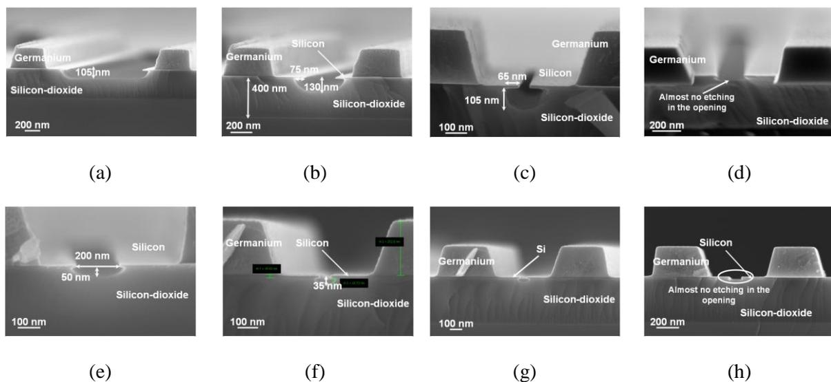
**Figure 9.** Cross-section SEM images after vapor phase hydrofluoric acid (VHF) etching for samples implanted with (a) and (e) Arsenic, (b) and (f) Phosphorous, (c) and (g) Boron and (d) and (h) unimplanted. VHF etching is carried out in a sequence of etch and rinse cycles at 55°C for (a)-(d) and at 75°C for (e)-(h), respectively.
