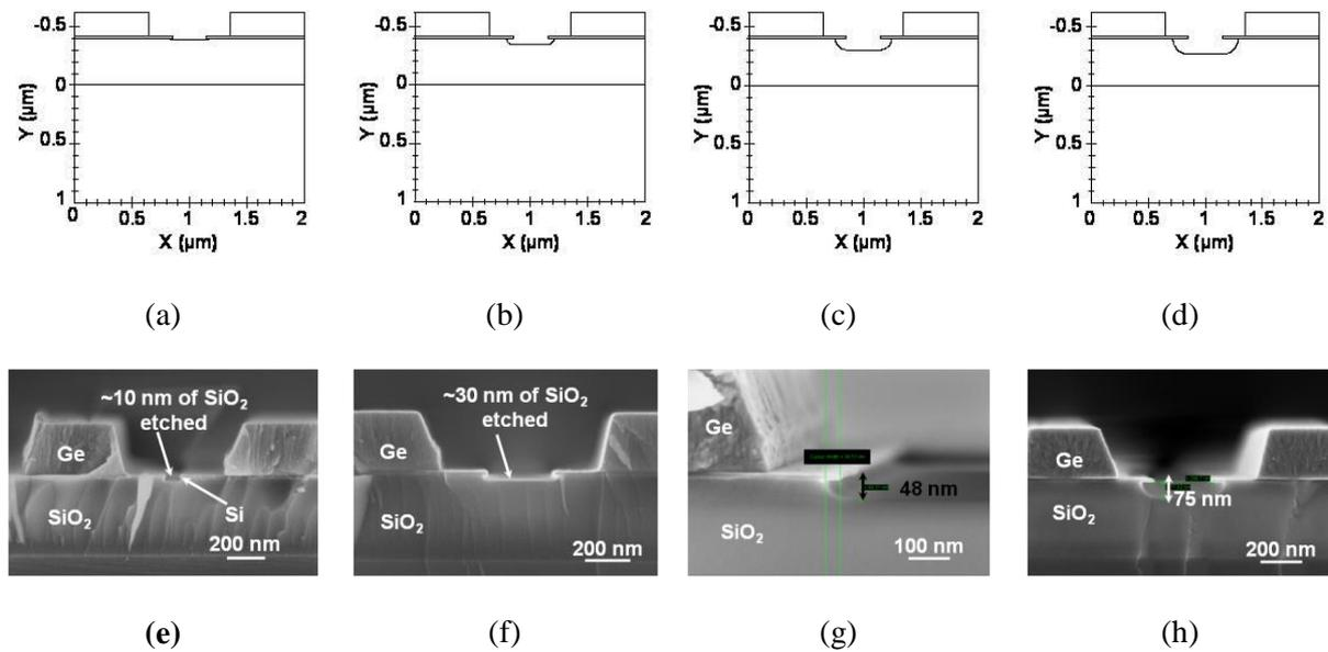
**Figure 7.** Simulated profiles of unimplanted silicon dioxide etched with HF-1% for various time (a) 2 mins, (b) 5 mins, (c) 10 mins and (d) 15 mins. (e)–(h) show the cross section SEM micrographs of the
