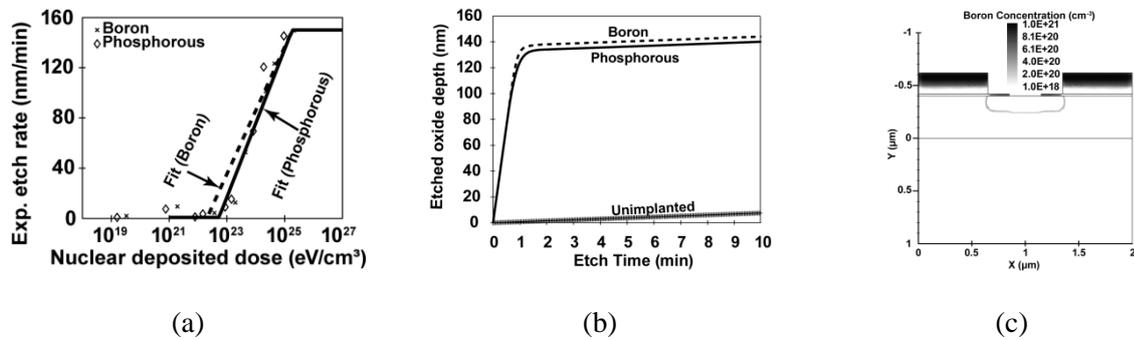
**Figure 8.** (a) Simulation profile nuclear deposited dose as a function of experimental etch rate of implanted silicon-dioxide using VHF for Boron and Phosphorous (Arsenic not shown), (b) Etched oxide depth as a function of etch time. The graph shows clearly the enhancement in etch rate of the implanted silicon-dioxide when compared to the unimplanted silicon-dioxide, (c) 2-D implantation profile of Boron implanted silicon-oxide after VHF etch.
