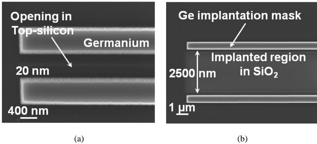
**Figure 4.** Top-view SEM images of Ge implantation mask on top of the patterned thin silicon layer, for the opening of (a) 20 nm and (b) 2,500 nm in the top Si layer. Openings in the germanium layer are regions in the silicon-dioxide which will be implanted.
