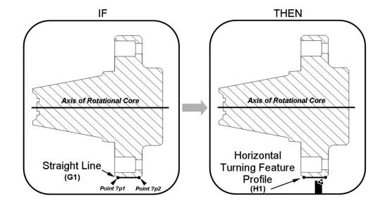
Example of a mapping rule for sharing between the rotational core design and manufacturing domains G3x35mm (600 x 600 DPI)
