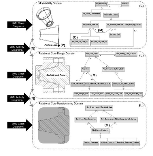
Using UML class and activity diagrams in the lightweight model 63x66mm (600 x 600 DPI)
