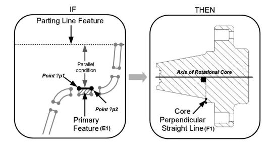
Example of a mapping rule for sharing between the mouldability and rotational core design domains 63x35mm (600 x 600 DPI)
