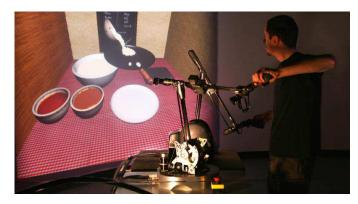
Fig. 12. The virtual crepe preparation simulator: the user pours some batter (a high viscosity fluid) from the bowl and into the pan. He feels the forces and torques from the pouring movement, as well as the weight shifting between his hands as the batter goes from the bowl to the pan.
