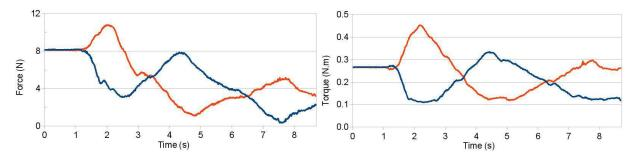
Fig. 11. Bimanual coupling on the same rigid body. Plot of the force (left) and the torque (right) generated by fluid inside a bucket coupled to two 6DoF haptic devices (left hand in red/light, right hand in blue/dark). The peaks and valleys correspond to the tilting movements, increasing the force and the torque on the side to which the bucket is tilted. Forces and torques progressively decrease as fluid is spilled.
