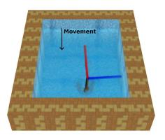
(a) Force (in red) and torque (in blue) exerted on the spoon. The force is opposite to the spoon movement. The torque shows a clock-wise effort in accordance to the spoon movement.
