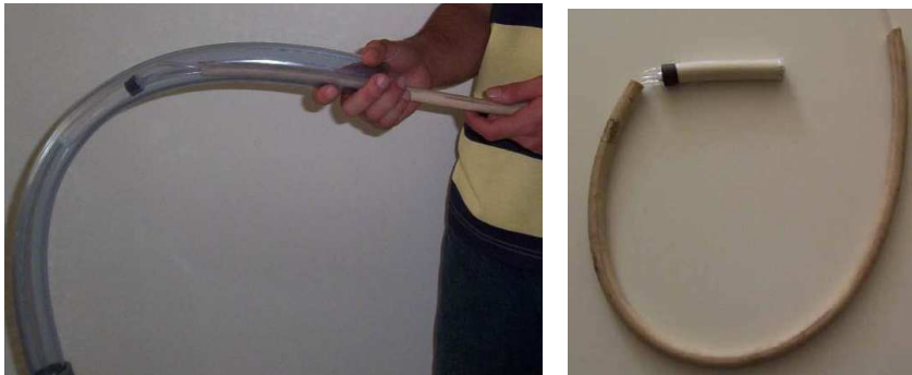
Fig. 25. Guidance control test in a colon-like tube
