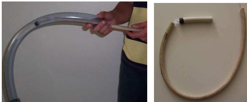
Fig. 25. Guidance control test in a colon-like tube
