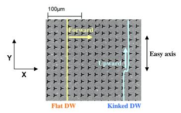
**Figure 1** (colour online) SEM micrograph of a square array of arrow holes. Solid lines are sketches of a flat and a kinked DW. Arrows indicates forward DW propagation sense and upward kink propagation sense. Note that Upward kink propagation is equivalent to net backward DW motion.
