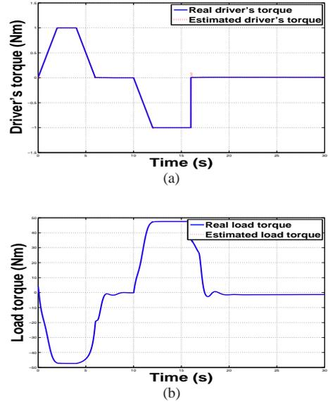
Fig. 7. (a) Real driver's torque (solid) vs. estimated driver's torque (dotted). (b) Real load torque (solid) vs. estimated load torque (dotted).
