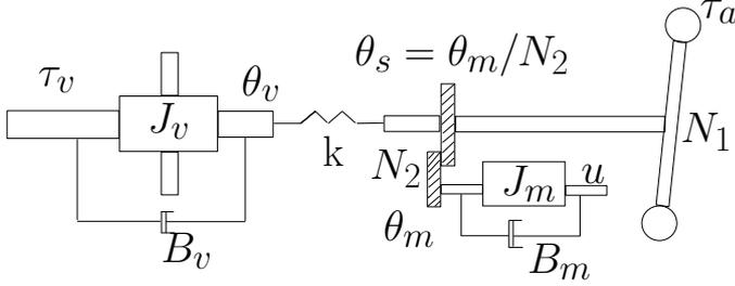
Fig. 2. Mechanical model of the EPSS
