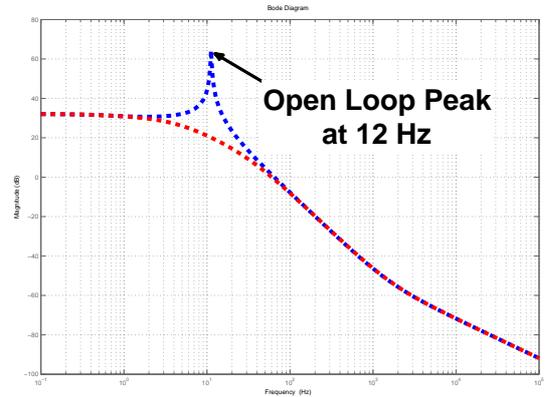
Fig. 3. Open loop (blue) vs closed loop frequency response. Weighting parameters are:  $q_1 = 3$  and  $q_2 = 12$ ,  $r = 1$ .
