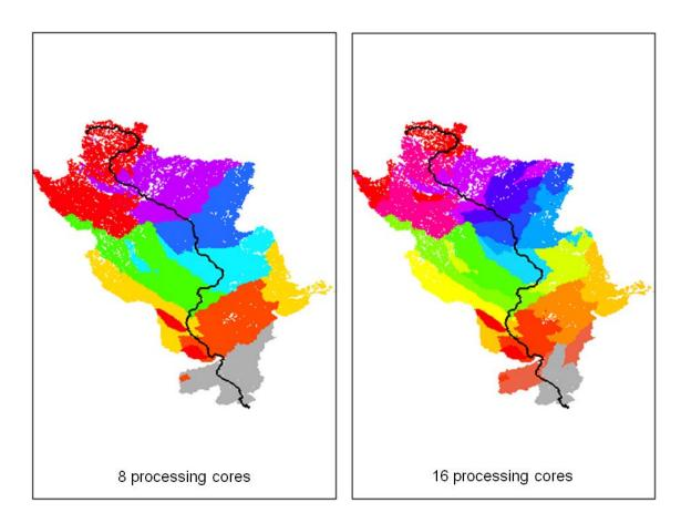
Figure 13 Longest path in the Upper Mississippi River Basin and location of sub-basins when RAPID is used in a parallel computing environment with 8 and 16 processing cores, different colors correspond to different cores.
