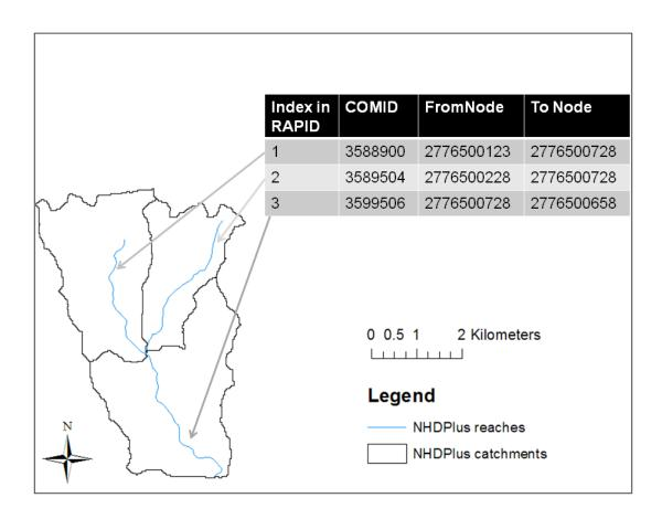
Figure 14 NHDPlus connectivity between reaches, nodes and catchments
