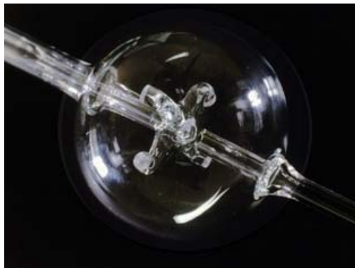
Figure 2. A perfectly stirred quartz reactor.
