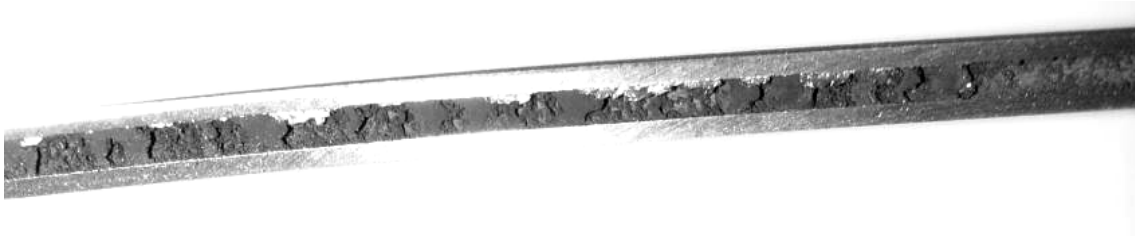
Figure 5. Stainless steel reactor, of 1.8 \cdot 10^3 m inner diameter, jammed by coke.
