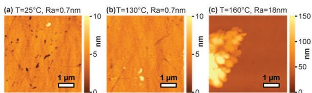
**Fig. 4** AC-AFM images of a vacuum-deposited thin-film of **1** ( $5 \times 5 \mu\text{m}$ ): non-heated film (a). Film heated (1 h) in air at  $130^\circ\text{C}$  (b) and  $160^\circ\text{C}$  (c).
