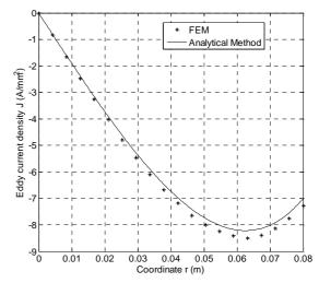
Fig.10. Eddy current density versus the radial distance r (at z=0) for  $V=0.62~{\rm m/s}$  and  $J=200~{\rm A/mm^2}$
