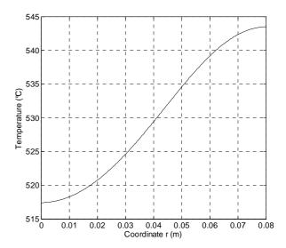
Fig.20: Temperature distribution in the billet versus the radial distance r for V=0.62 m/s and J=200 A/mm<sup>2</sup> at time t=150 s.
