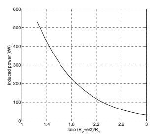
Fig.18. Eddy current versus the distance between the inductor and the billet for V = 0.62 m/s and J = 200 A/mm<sup>2</sup>
