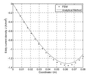
Fig.9. Eddy current density versus the radial distance r (at z=0) for  $V=0.24~{\rm m/s}$  and  $J=200~{\rm A/mm}^2$
