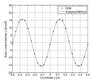
Fig.11. Eddy current density versus the axial distance z (at  $r=R_I$ ) for  $V=0.24~\mathrm{m/s}$  and  $J=200~\mathrm{A/mm^2}$
