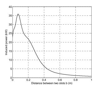
Fig.15. Induced heating power versus the distance between two superconducting coils for V = 0.24 m/s and  $J = 200 \text{ A/mm}^2$
