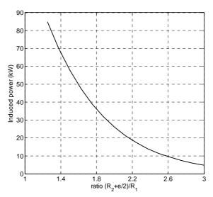
Fig.17. Induced power versus the distance between the inductor and the billet for V = 0.24 m/s and J = 200 A/mm<sup>2</sup>
