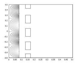
Fig.7. Eddy current distribution in the billet for  $V=0.24~\mathrm{m/s}$  and  $J=200~\mathrm{A/mm^2}$
