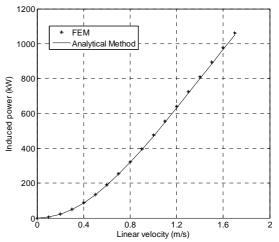
Fig.14. Induced heating power versus the linear velocity for  $J = 200 \text{ A/mm}^2$
