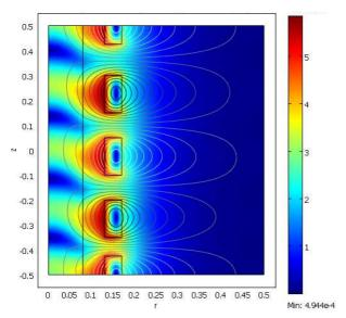
Fig.6. Flux lines distribution and magnetic flux density distribution (T) for V = 0.62 m/s and  $J = 200 \text{ A/mm}^2$
