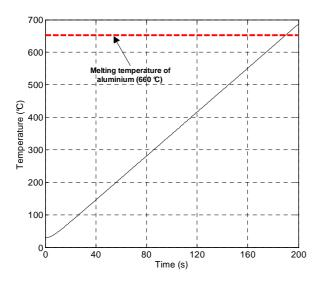
Fig.19: Transient temperature profile at the center of the billet for V=0.62 m/s and J=200 A/mm<sup>2</sup>
