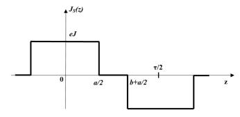
Fig.3. Current sheet distribution along the axial coordinate z
