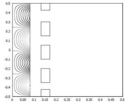
Fig.8. Eddy current distribution in the billet for V = 0.62 m/s and J = 200 A/mm<sup>2</sup>.
