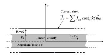
Fig.2. Simplified model used for the analysis
