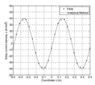
Fig.12. Eddy current density versus the axial distance z (at  $r=R_I$ ) for V=0.62 m/s and J=200 A/mm<sup>2</sup>
