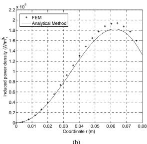
Fig.13. Induced power density versus the radius r at z=0 a) V=0.24 m/s b) V=0.62 m/s
