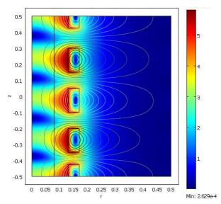
Fig.5. Flux lines distribution and magnetic flux density distribution (T) for V = 0.24 m/s and  $J = 200 \text{ A/mm}^2$
