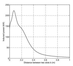
Fig.16. Induced heating power versus the distance between two superconducting coils for  $V=0.62~{\rm m/s}$  and  $J=200~{\rm A/mm^2}$
