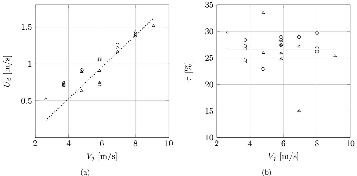
**Figure 3.** Measured doppler velocity  $U_d$  (3(a)) and turbulence intensity  $\tau$  (3(b)) as a function of the nozzle velocity  $V_j$  at 2.3 K ( $\Delta$ ) and 2.0 K ( $\circ$ ). The dotted line ( $\cdots$ ) and the solid line ( $\text{---}$ ) represent the expected mean velocity on the jet axis at 30 diameters downstream (Hussein *et al.*, 1994) and the mean of the turbulence intensity, respectively.
