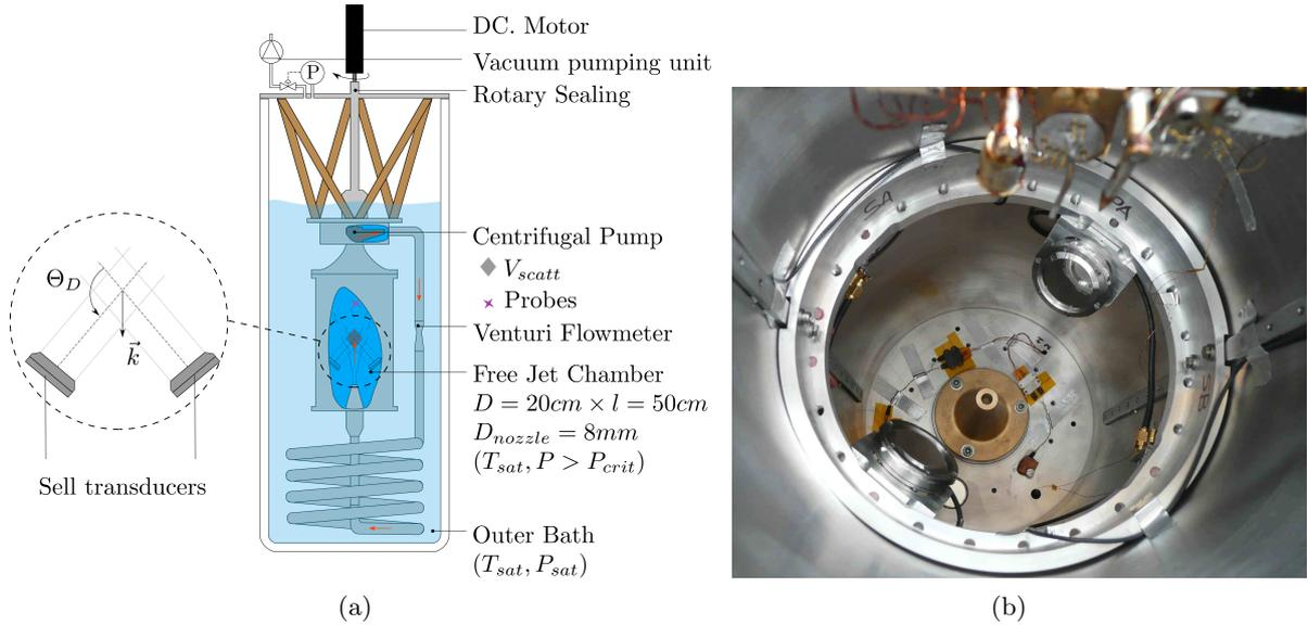
**Figure 1.** Schematic drawing 1(a) of the cryogenic wind tunnel testing facility (not in scale). The enlarged view shows the ultrasound acoustic scattering set-up geometry. 1(b) shows a photograph of the transducers and the nozzle, taken from the top of the test chamber.
