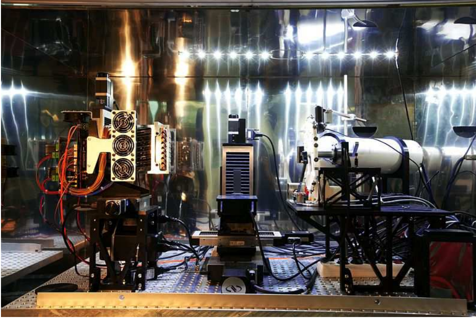
Figure 3: Picture of the PIXSCAN II scanner with the three distinct blocks. From left to right : the XPAD3 detector block, the imaged object block, and the source block.
