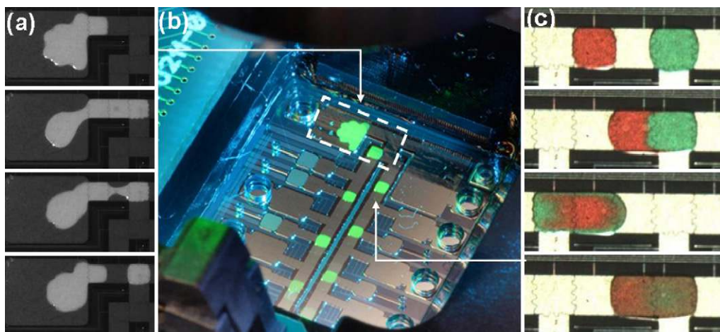
Fig. 1. Assembly of pictures illustrating basic operations on EWOD chip devoted to biological protocols: (a) drop on demand from a liquid tank with a CV < 3%. (b) Several droplets are displaced from one electrode to the other. (c) Mixing with two colored droplets merged and moved back and forth.
