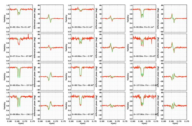
**Fig. 3.**  $\alpha$  Col differential visibility and phase from our four VLTI/AMBER HR measurements (red line). Each row corresponds to one VLTI/AMBER measurement (three different baselines). The visibility and phase of the best-fit kinematics model is overplotted in green.
