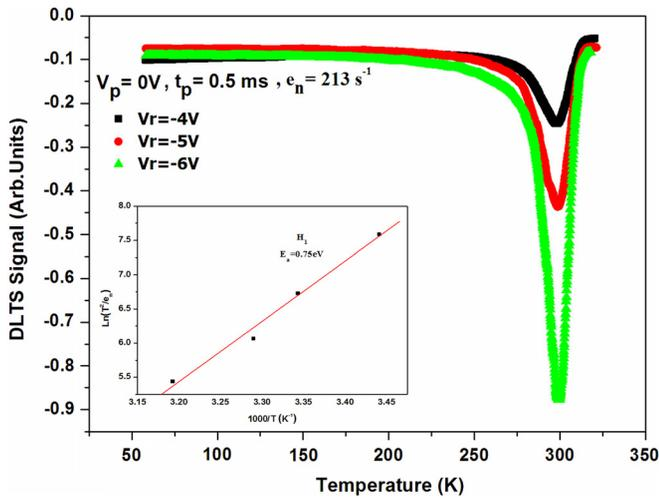
FIG. 10. (Color online) DLTS spectra measured with a reverse bias of  $-4$  V,  $-5$  V and  $-6$  V, a pulse filling time of  $0.5$  ms and for an emission rate ( $e_n$ ) of  $213$   $s^{-1}$ . The inset shows the Arrhenius diagram for the  $H_1$  hole trap observed in the (Ni/Au)/AlGaIn/GaN/SiC SBD with DLTS measurements.
