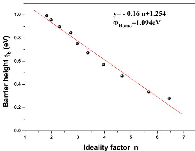
FIG. 3. (Color online) Plot of  $\phi_b$  vs  $n$  showing a linear correlation between these parameters; the extrapolation at  $n = 1$  gives a value of the homogenous barrier  $\phi_{\text{Homo}} = 1.094$  eV.
