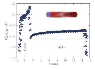
FIG. 9. (Color online) VB edge in a GaAs-quantum-dot/AlAsquantum-rod heterostructure (diameter of the core sphere and of the cylindrical rod d = 3.2 nm; total length l = 17.2 nm). For clarity, only atoms with r < 1.2 nm are plotted, where r is the distance to the symmetry axis. The dashed horizontal lines indicate the VB offset in the 2D GaAs/AlAs superlattice.
