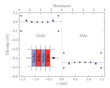
FIG. 1. (Color online) VB edge in a  $(GaAs)_8(AlAs)_8$  (110) superlattice. The average potential in the GaAs layer has been shifted to zero, so that the horizontal dashed lines directly indicate the VB offset.
