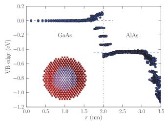
FIG. 2. (Color online) VB edge in a spherical GaAs/AlAs core/shell quantum dot as a function of the radial position of the atoms (core diameter  $d_c = 4$  nm; shell diameter  $d_s = 7$  nm). The horizontal dashed lines indicate the VB offset in the 2D GaAs/AlAs superlattice.
