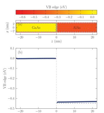
FIG. 7. (Color online) (a) 2D plot of the VB edge in a section of a GaAs/AlAs nanowire superlattice surrounded by an AlAs shell (core diameter  $d_c = 5$  nm, shell diameter  $d_s = 6$  nm; length of each GaAs or AlAs segment l = 22.5 nm). (b) VB edge along the axis of the nanostructure. The horizontal dashed lines indicate the VB offset in the 2D GaAs/AlAs superlattice.
